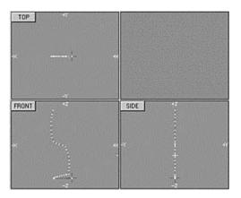
When you are satisfied with the outline, position the 3D cursor in the Top view window. The Top window will now be the active one and is highlighted with a yellow border. The axis of spin of the lathe will therefore be at right angles to the Top window, that is, up/down or in the direction of the Z axis.
