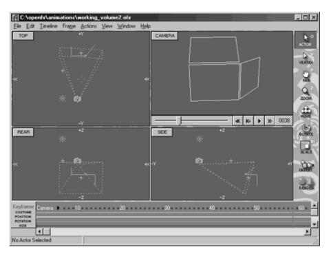
The visible region of the world is inside a cubic volume known as the <u>Working-Volume</u>. The Working-Volume may be moved through space and changed in size.
